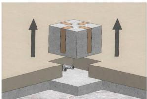
Place for floor socket/ First set up box, made from polystyrene or formwork (size should be 2-4 cm bigger than corresponding box for floor socket. After pouring concrete, remove polystyrene.
