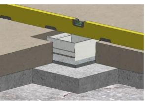
Insert pipe/s with wires into set holes (25mm). Attached end caps Ø25 are for unused hole. This end caps can be used as bushing (need to drill holes into it) for specific wires, it's possible to take out socket holder (including sockets) to prevent any damage during install. Floor box is pushed by water level into mortar/glue basis. Upper edge of the box should be levelled with concrete
