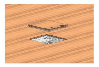
Cut the lid from floor material (Be careful about wood patterns!), size 220x150mm or depends on size of the hole made for the box. Glue aluminium lid (210x140mm) to the lid from floor material; be sure it's glued in the centre. Cut openings in relevant places for electric cords. If multiple holes not needed, you don't have to cut them out)
