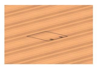
4 spacing screws, which are always located in the corner of the box, allow for a slight (approx. 5 mm) adjustment of the lid height (lid lifting) so that the lid is in the same plane as the floor covering around the floor box.
