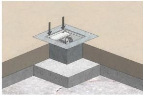
Rest of the empty space around floor box is filled by glue/mortar etc. Fill it to the same level as surrounding concrete floor. Prepared wires will connect to corresponding sockets and socket holder is inserted back.
